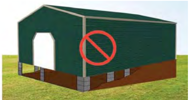
No Installs on Unlevel Land
