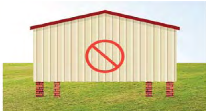
No Installs on Stacked Blocks
